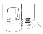
Pressing the MUTE button turns off the microphone during a telephone conversation at the speakerphone and the intercom so that you may speak to someone in the room with you without the caller overhearing. The SP/INTCOM LED will blink in this mute mode. Press the SPEAKERPHONE button or MUTE button again to resume normal conversation.
