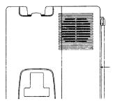
You can select and adjust the ringer volume. For no ring at all, slide the switch to the OFF position when the handset is off the base unit. Note that the handset will ring regardless of which position you have selected.
