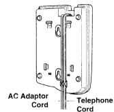
4 Place the base's keyhole slots over the two screws and gently push down on the base unit to lock it into place.
