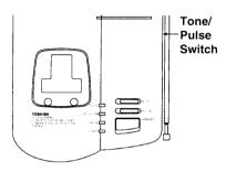
Set the TONE/PULSE switch located on the side of the base unit for the type of service you have (tone or pulse). If you are not sure which type of service you have, do this simple test.
